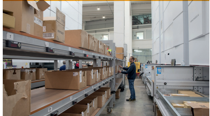
Put-to-Light systems connected to WMS
