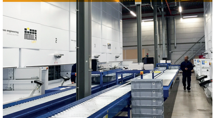
Integration with conveyors
