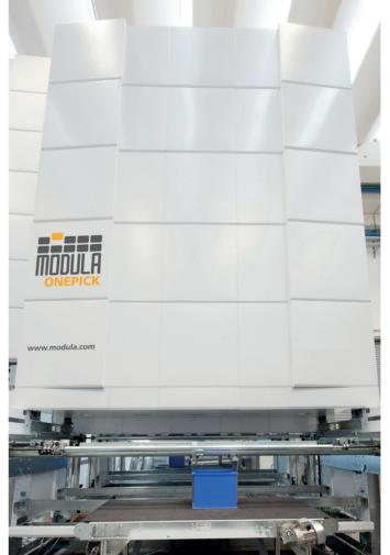
Maximum load unit height: 360 mm
